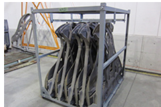
Returnable packing rack for grand piano frames
