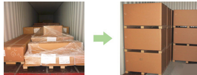
Loading container with pre-standardization packing boxes (left) and loading container with standardized packing boxes (right)
