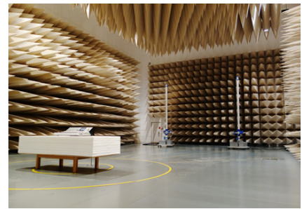
Anechoic chamber used for electromagnetic wave measurement
