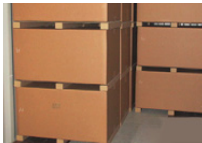
Loading container with pre-standardization packing boxes (left) and loading container with standardized packing boxes (right)
