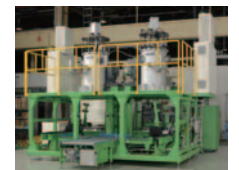
Helium leak tester
