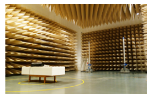
Anechoic chamber used for electromagnetic wave measurement
