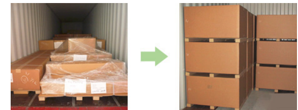
Loading container with pre-standardization packing boxes (left) and loading container with standardized packing boxes (right)
