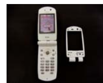
Molded with magnesium alloy
